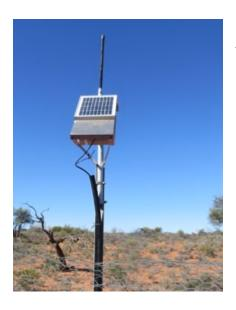
One of the new telemetry signal boxes set up at the Arid Recovery Reserve.
