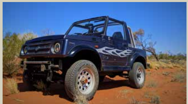
Arid Recovery's electric 4WD converted Suzuki ute
